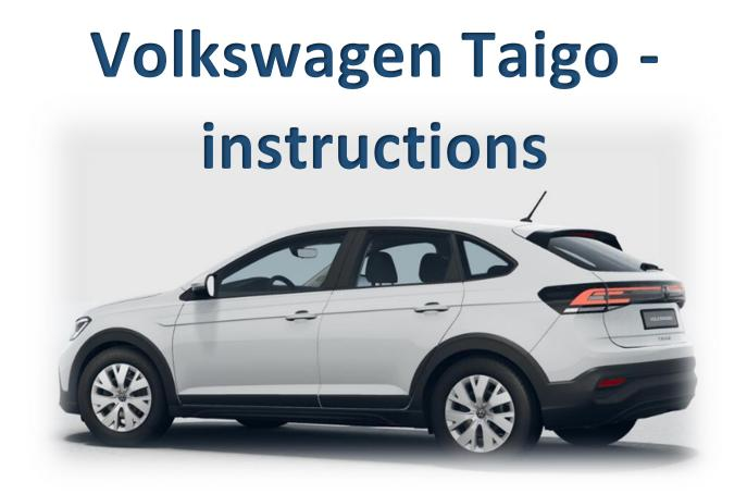
Volkswagen Taigo, 1,0 TSI, ym. 2024 Engine: 999cm<sup>3</sup>, 3 cylinder, turbo Gearbox: manual 5 gears Top power: 70kw (95hp) /6500rpm Top torgue: 175nm /4500rpm Weight:: 1229 kg Fuel consumption:: 5,4 l/100km WLTP CO2 Emissions: WLTP CO2 122g/km
